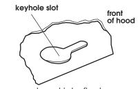
Lift the range hood into final position and center. Mark on the underside of cabinet the location of the four keyhole mounting slots. Set range hood aside on a protected surface.
